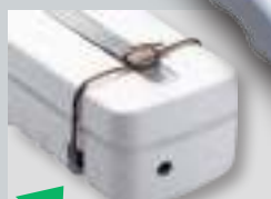
fig. 3: Material thickness compensator with material sample inserted
