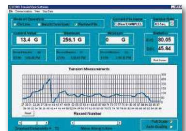
fig. 4: Model DTMX provides detailed process data and analysis (for software see page C 9)
