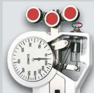
fig. 1: Adjustable damping (Code A) to provide steady tension readings (see page F)
