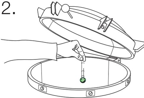
*Place one capsule (or 2 if the odor is strong) in the water at the bottom of the autoclave.*
