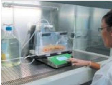
New standards make it necessary to work under a laminar flow for the dilution work, and this can create operational problems.
